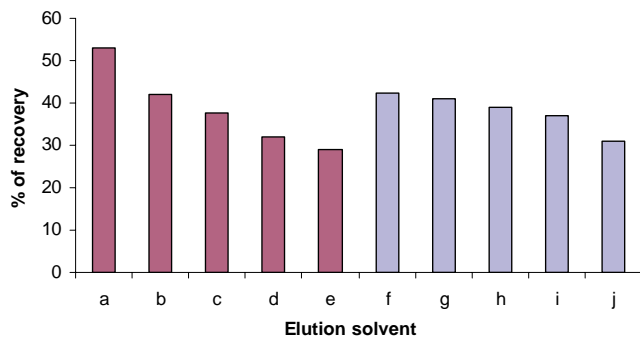
Fig. 7. Recovery of compound A using MIP2 with various elution solvents. Solvents a–e contained methanol with (a) 2% TFA, (b) 5% ammonia, (c) 5% triethylamine, (d) 5% formic acid and (e) 0.1 M HCl. Solvents f–j contained 2% TFA in (f) acetonitrile, (g) acetonitrile/methanol/water 60/35/5 (v/v/v), (h) THF/water 70/30 (v/v), (i) acetonitrile/water 70/30 (v/v) and (j) methanol/water (v/v).
